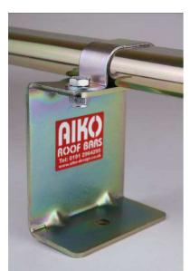
You can probably see what's coming next-lay your cross bars across the tops of your brackets, drop a strap over the top and put in the M6 bolts, with a washer and Nyloc nut underneath; don't tighten things fully yet though as first we need to add the longitudinal bars. (Plain for RS customers, and with the raised sides on the FS set-FS shown)
